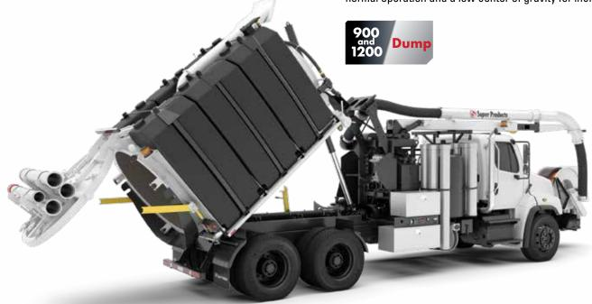
**Ejection Unloading:** The ejection unloading system is the industry's safest and most efficient removal of debris. The body raises to an 8.5° angle and the ejector plate quickly pushes out debris. This allows operators to have **the only controlled way to dump into a 48-inch container** without the need of additional containment products.
